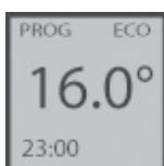
If the screen displays PROG ECO, you are in a programming range in ECO mode. To modify the ECO range temperature, use the ECO Temp. menu (see "The menu in PROG mode" chapter).
