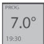
If you set a Frost Protection temperature (7°C) when you changed to the programming range in ECO mode, the screen displays 6°.0 (automatic 1°C drop).
