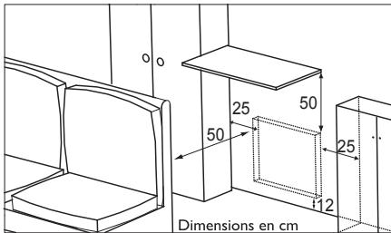
Comply with the minimum clearance distances for positioning of the device.
